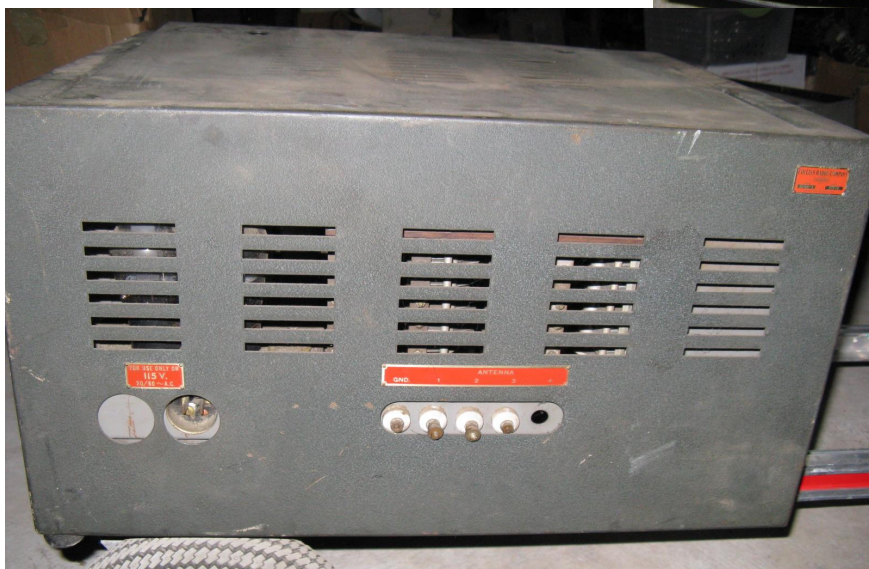
Collins Type 32RA 1.5 -15 Mhz 75 watt transmitter, coils are included
